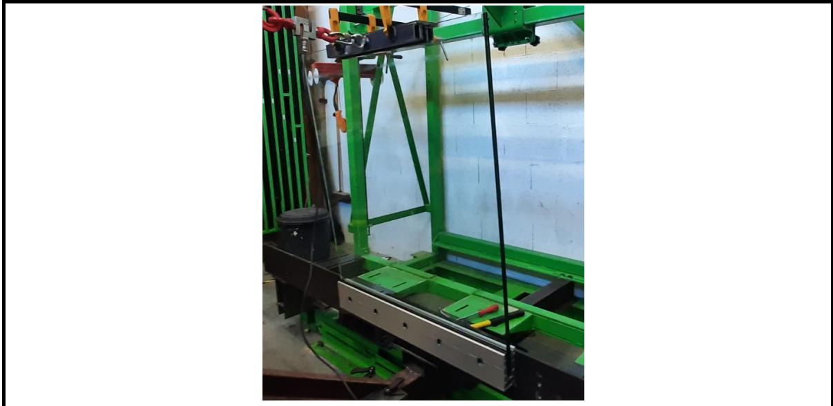
Railing under imposed load Pe
